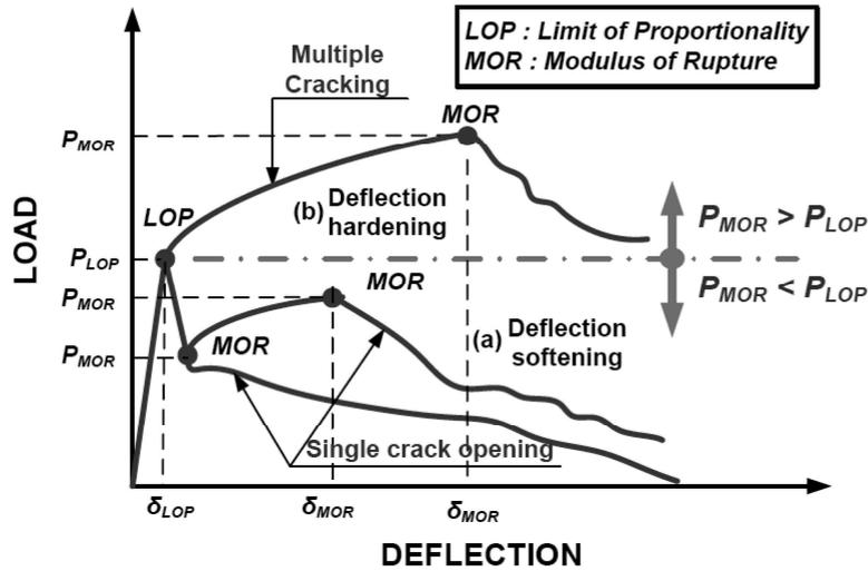
Fig. A.3.6.1 Typical load-deflection curves of K-UHPC under flexural tension stress
