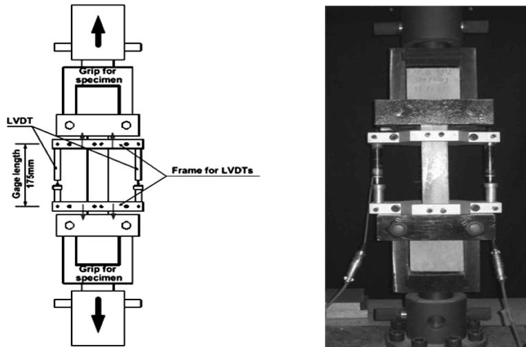
Fig. A.4.5.1 Direct tensile strength test of K-UHPC (unnotched specimen)
