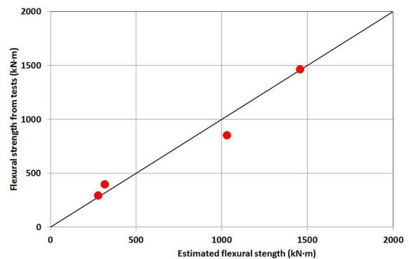
(b) Test results for T-shape beam
