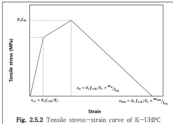
Fig. 2.5.2 Tensile stress-strain curve of K-UHPC
