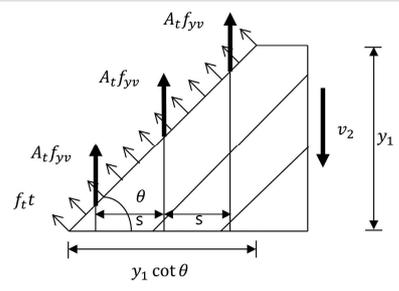
**Fig. c.7.3.3** Shear force of second surface of equivalent thin-walled tube
