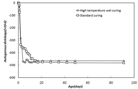
Fig. c.2.9.3 Autogenous shrinkage of K-UHPC
