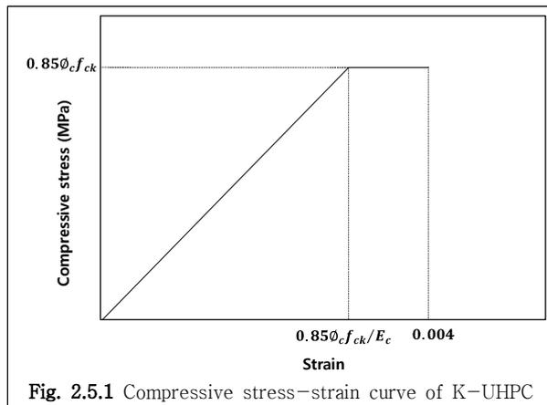
(2) The idealized compressive stress-strain curve presented in Figure 2.5.1 can generally be used for the examination of the section forces at the ultimate state of a member subjected to flexural moment or simultaneously to flexural moment and axial compressive force. In such case, the material reduction factor  $\phi_c$  is set to 0.91 and the elastic modulus  $E_c$  is determined with respect to Section 2.6. In addition, the design compressive strength  $f_{cd}$  becomes  $\phi_c f_{ck}$ .
