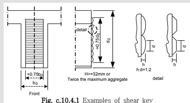
Fig. c.10.4.1 Examples of shear key
