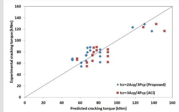
Fig. c.7.3.2 Comparison of cracked torsional moment of K-UHPC beam
