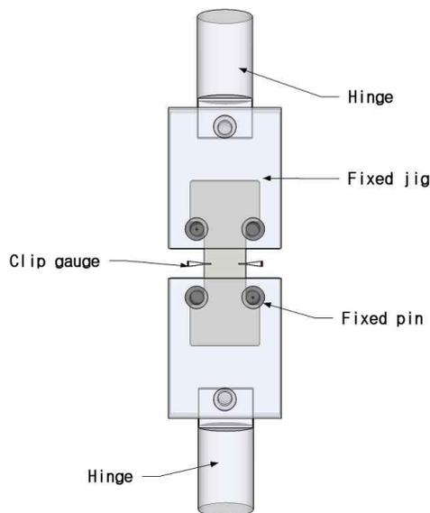
Fig. A.5.5.1 Direct tensile strength test of K-UHPC (notched specimen)
