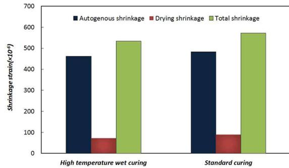
Fig. c.2.9.1 Shrinkage strain of K-UHPC
