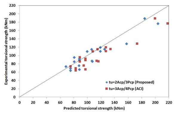
**Fig. c.7.3.5** Comparison of ultimate torsional moment of K-UHPC beam
