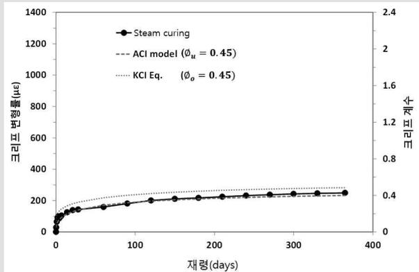
Fig. c.2.10.2 Creep test results for high temperature wet curing condition
