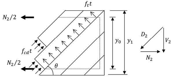
**Fig. c.7.3.4** Longitudinal force of second surface of equivalent thin-walled tube
