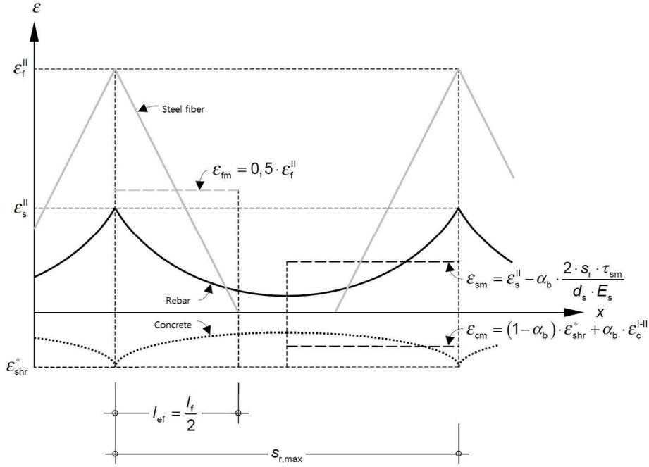
Fig. A.6.2.1 Strain of reinforcement, steel fiber and concrete in steady state cracking
