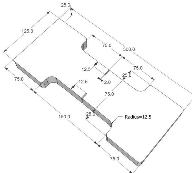
Fig. A.1.5.2 Notched specimen for direct tension (unit: mm)
