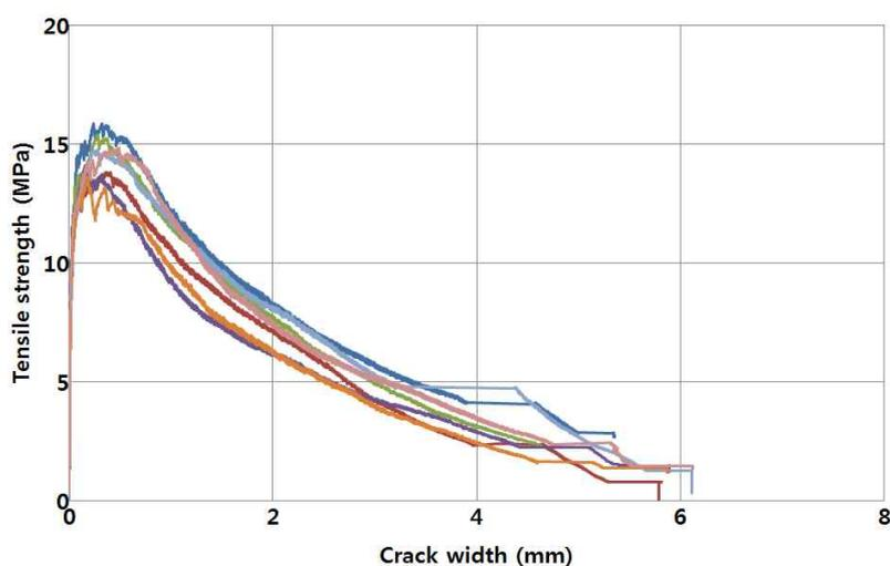
Fig. A.5.6.1 Tensile stress-opening displacement curve
