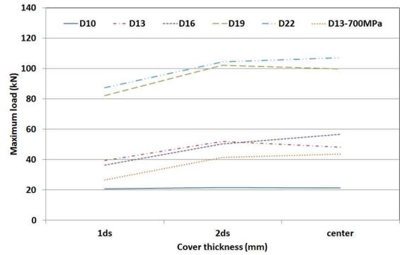
Fig. c.5.2.1 Variation of peak load sustained by rebar according to cover thickness
