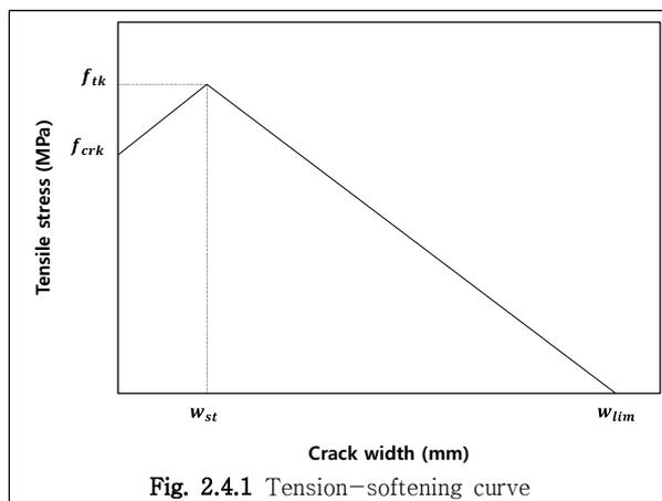
In Figure 2.4.1,  $w_u$  designates the crack width at tensile strength caused by strain-hardening after the initiation of crack and,  $w_{lim}$  stands for the crack width at which tensile stress vanishes.
