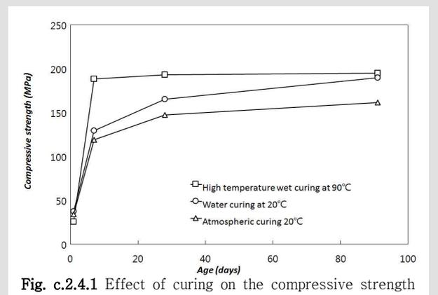
Fig. c.2.4.1 Effect of curing on the compressive strength
