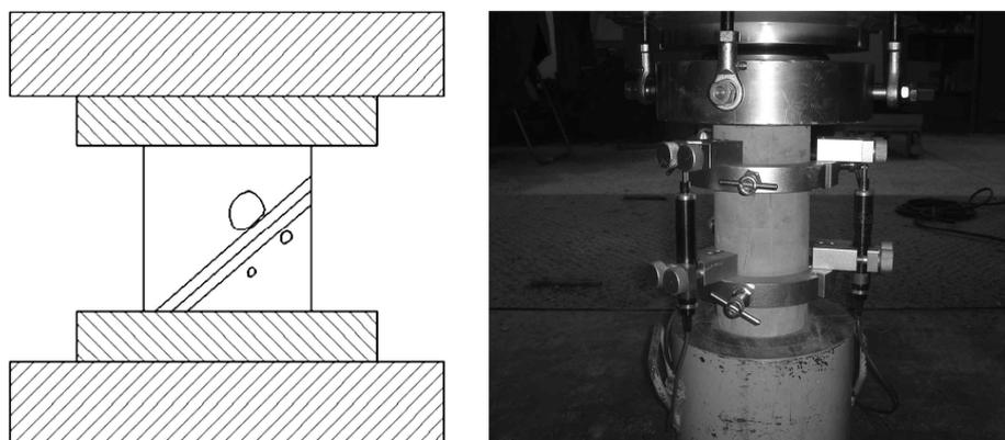
Fig. A.2.4.1 Compressive strength test of K-UHPC
