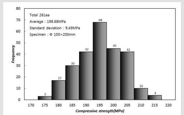
Fig. c.2.4.2 Frequency distribution of compressive strength resulting from strength test on 100 mm-diameter cylinders
