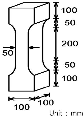
Fig. A.1.5.1 Unnotched specimen for direct tension
