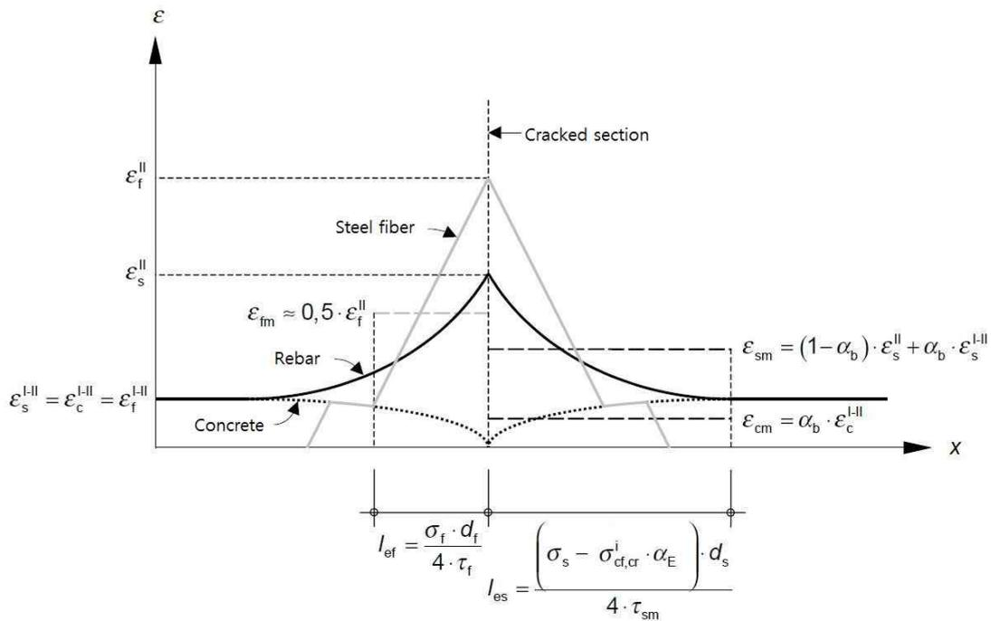
Fig. A.6.1.1 Strain of reinforcing bar, steel fiber and concrete under single crack state
