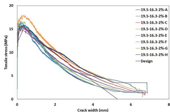
**Fig. c.2.4.3** Characteristic tensile stress–crack width curves obtained by direct tensile test
