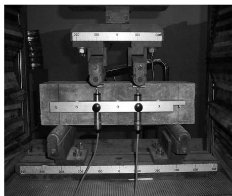
Fig. A.3.4.1 Flexural strength test of K-UHPC
