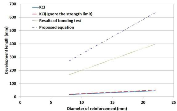
Fig. c.8.2.1 Development length of K-UHPC according to the diameter of reinforcement
